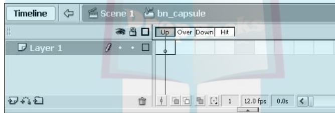
Figure 8-2: The Flash symbol-editing mode for buttons displays a Timeline with four frames.
